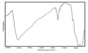
Fig. 2. FTIR spectrum of Tin(IV) tungstoselenate
