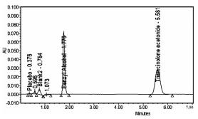
Fig. 8. Oxidative degradation sample chromatogram at 215nm
