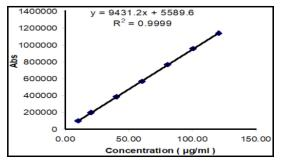
Fig. 13. Triamcinolone acetonide Linearity graph The Limit of detection and quantitation
