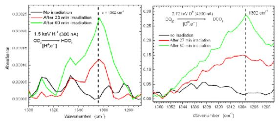
Fig. 6(a-b): Shows tentative signals for  $H_2CO_3$  and  $D_2CO_3$  - both at v = 1302 cm<sup>-1</sup>. However, it should be noted that, in general, the presence of  $D_2$  in  $D_2CO_3$  should produce a slightly different vibrational mode from v = 1302 cm<sup>-1</sup>
