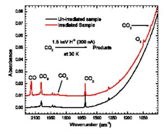
Fig. 3: Shows the displaced spectra, illustrating the formation of new species of molecules during the irradiation of  $CO_2$  ice at 30 K and using 1.5 keV H<sup>+</sup> ions
