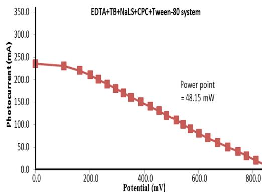
**Fig. 3. Cell Performance (i-V) curve for three mixed surfactants****Table 2: Indicates that the diffusion lengths (DL) of the three substances vary**
