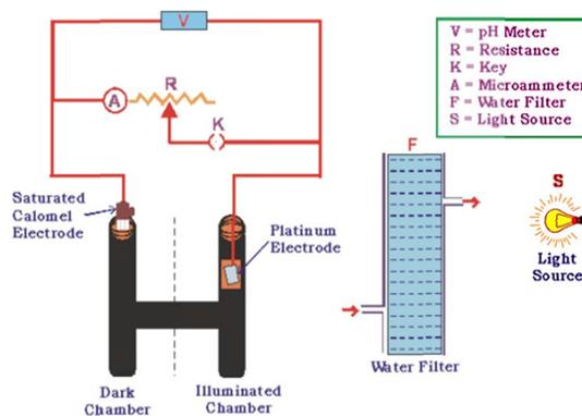
Fig. 1. PG Cell for three mixed surfactants
