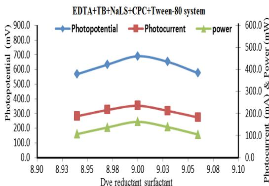
**Fig. 2. Electrical output for three mixed surfactants****Variations in EDTA concentration and their effects**
