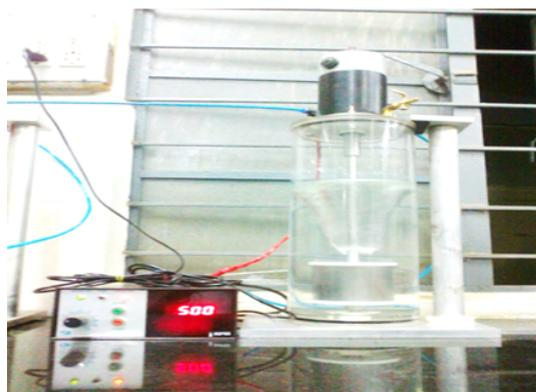
Fig. 1(c). Rotating cage at 500 rpm
