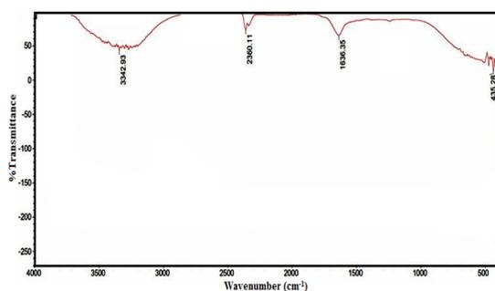
Fig. 2. FTIR spectrum of SrO NPs
