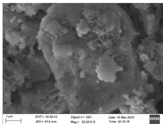
Fig. 4. SEM images of SrO NPs at  $1\mu\text{m}$  Crystallographic Analysis
