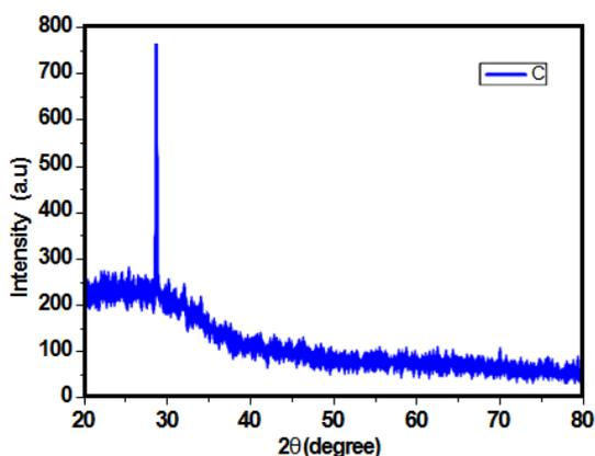
Fig. 5. XRD of strontium oxide nanoparticles
