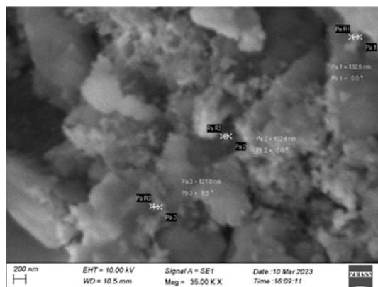
Fig. 3. SEM images of SrO NPs at 200 nm
