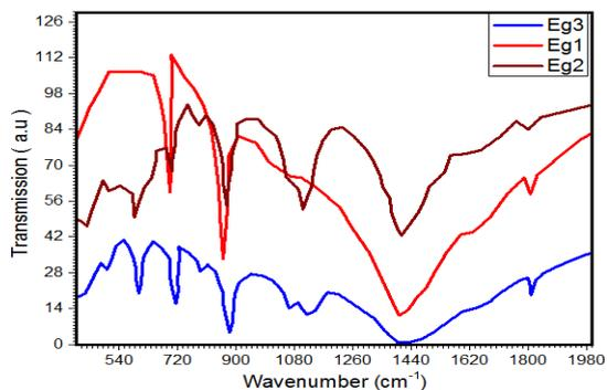
Fig. 2. FTIR result of natural Eg1, Functionalized egg-shell Eg2 and after removal copper Eg3
