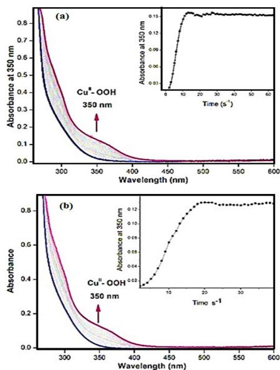
Fig. 3. The absorption spectra for the formation of hydroperoxy intermediates of complexes 1 (a) and 2 (b) (0.05 mM) with  $H_2O_2$  (0.5 mM) in carbonate buffer (0.1 M) at 30°C. Insert figures: Plot of  $1+Abs.$  vs Time
