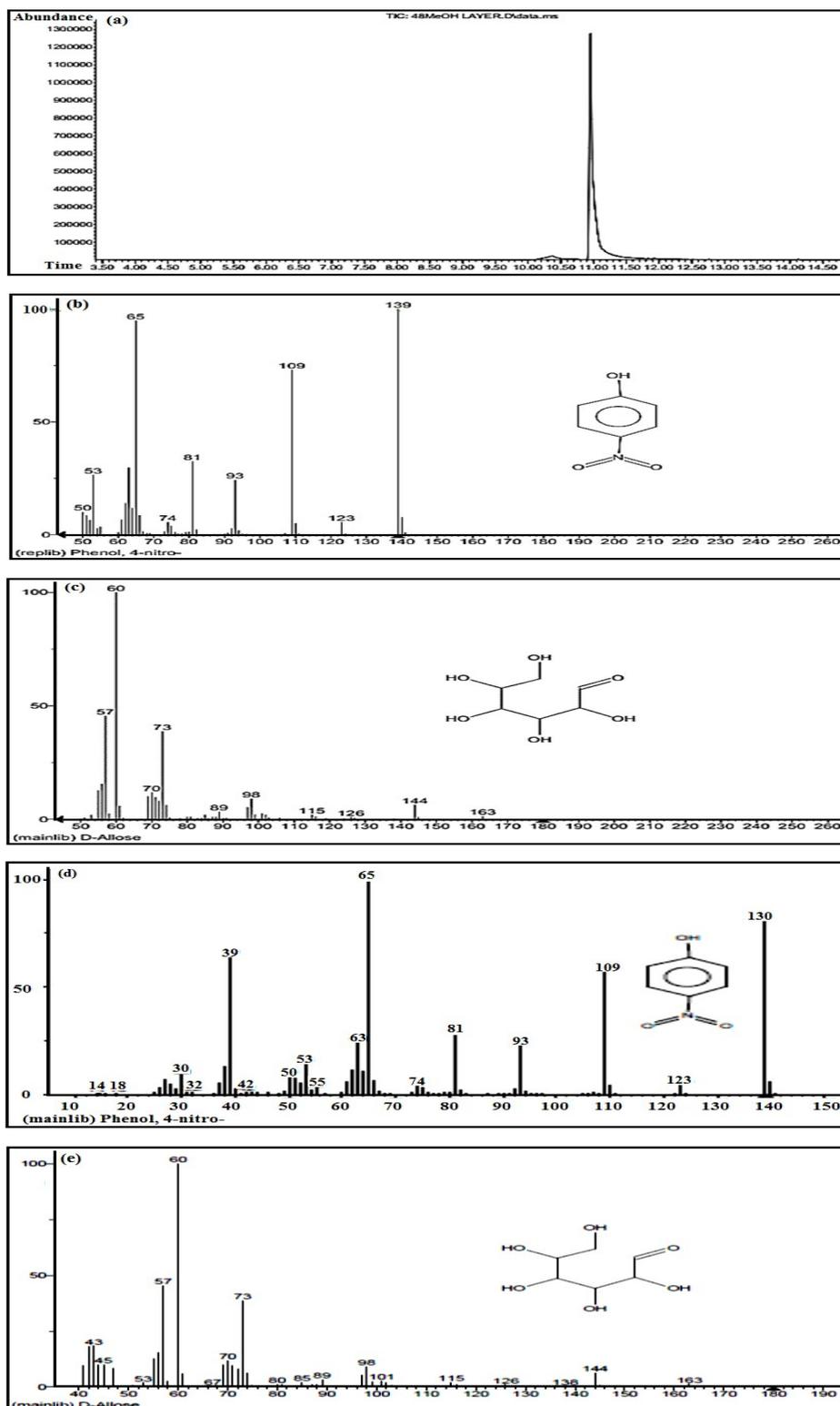
Fig. 7. GC-MS chromatogram of *p*-nitrophenyl- $\beta$ -D-glucopyranoside (a) and their respective products, *p*-nitrophenol (b) and D-allose (c). Authentic GC-MS spectra of *p*-nitrophenol (d) and D-allose (e)
