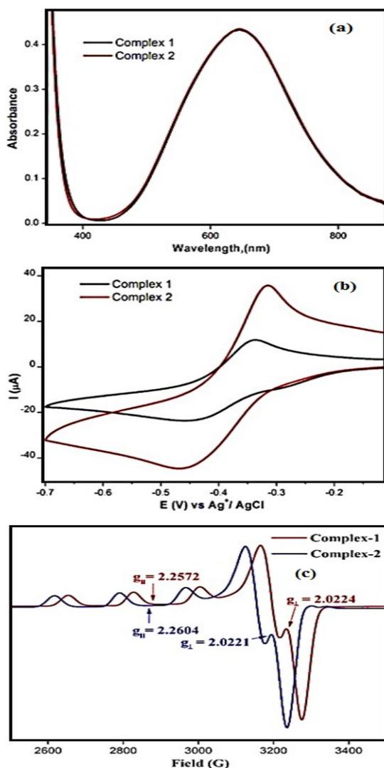
Fig. 2. Electronic spectra (a), cyclic voltammograms (b) and EPR (c) of complexes 1 and 2 ( $1 \times 10^{-3}$  M) in the presence of carbonate buffer at 25°C. The scan rate
