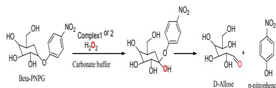
Scheme 2. Oxidative cleavage of  $\beta$ -PNPG and hydrogen peroxide with catalyst
