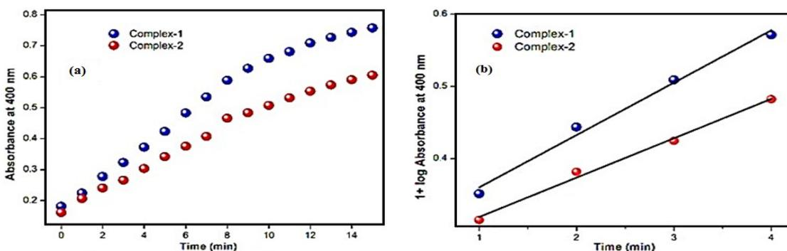
Fig. 5(a). Time dependent absorption spectra for the kinetic reaction of complexes **1** and **2** (0.05 mM) with the substrate (*p*-nitrophenyl- $\beta$ -D-glucopyranoside, 0.5 mM) in the presence of  $\text{H}_2\text{O}_2$  (0.5 mM), and (b) Plot of  $1 + \log(\text{Abs})$  vs Time in carbonate buffer (0.1M) at 30°C
