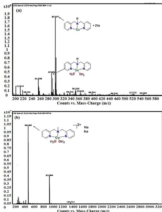
Fig. 1. ESI-MS spectra of complex **1** (a) and **2** (b) in methanol solution
