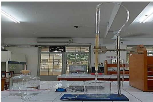
Fig. 1. Experimental setup for column dynamic adsorption
