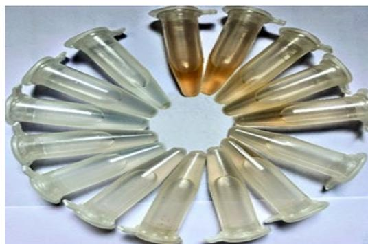
Fig. 7. Colorimetric results of CPTPH-AgNPs on addition of different amounts of L-Histidine
