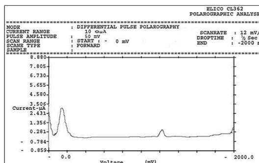
**Fig. 3. DC Polarogram and DPP Polarogram of salicylidene-4-(p-chlorophenyl)-2-aminothiazole (SCAT) ligand in B-R buffer at pH 7.4±0.01**
