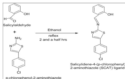
Fig. 1. Synthesis of salicylidene-4-(p-chlorophenyl)-2-aminothiazole (SCAT) ligand
