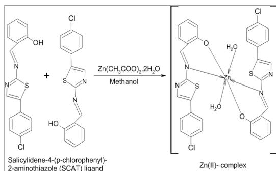
**Fig. 2. Synthesis of Zn(II)- salicylidene-4-(p-chlorophenyl)-2-aminothiazole (SCAT) complex**
