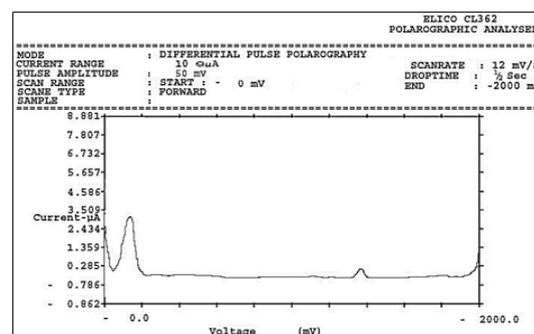
**Fig. 4. DC Polarogram and DPP Polarogram of Zn(II) Complex of salicylidene-4-(p-chlorophenyl)-2-aminothiazole (SCAT) ligand in B-R buffer at pH 6.5±0.01.**
