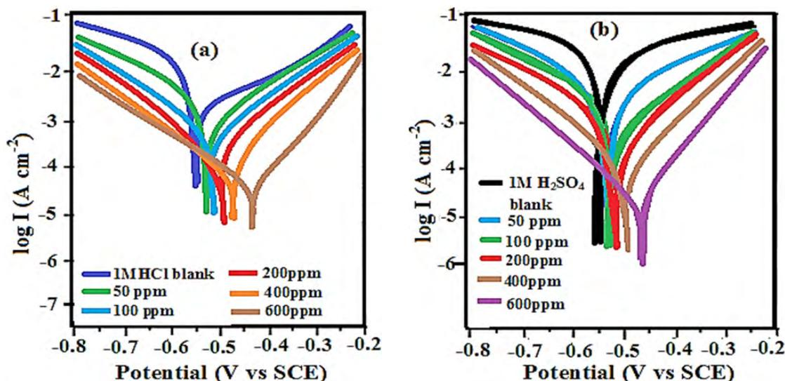
Fig. 6. Tafel plots of MS in NB4MA (a) 1M HCl (b) 0.5M H<sub>2</sub>SO<sub>4</sub>
