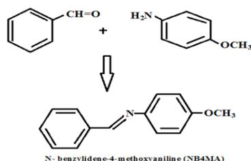
Fig. 1. Schematic diagram of synthesis of Schiff base NB4MA
