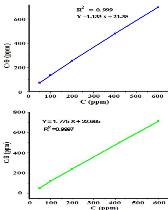
Fig. 9. Langmuir's isotherm of MS with NB4MA
