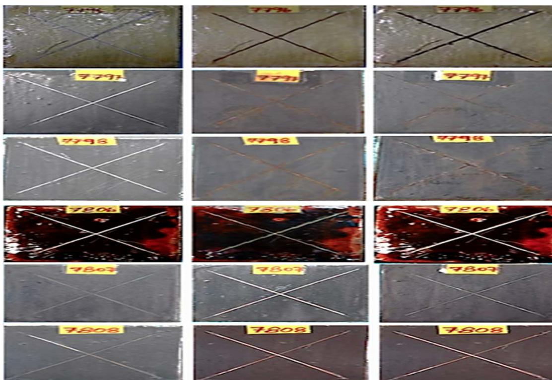
Fig. 4. Visual performances of salt spray test of mild steel and copper samples exposure to 5% NaCl solution at the initial time, after 144 and 300 hours. (a): Untreated epoxy /ms, (b) : GO-epoxy/ms, (c) : GO-KF-epoxy/ms (d): Untreated epoxy /Cu , (e) : GO-epoxy/Cu, (f) :GO-KF-epoxy/Cu
