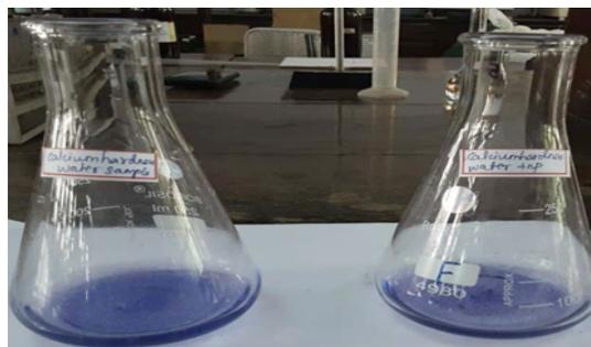
Fig. 4. Analysis of calcium hardness in tannery water
