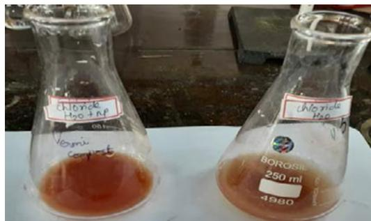
Fig. 5. Analysis of chloride in tannery water
