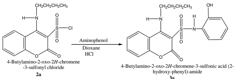
**Scheme 3: Synthesis of 4-Butylamino-2-oxo-2H-chromene-3-sulfonic acid (2-hydroxy-phenyl) -amide (3a)**
