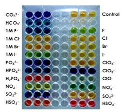
Fig. 1. Microplate wells containing 0.1 M anion solutions (unless otherwise indicated) in distilled water with a universal pH indicator solution. Tests were done in triplicates
