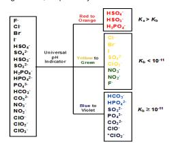
Fig. 2. Diagram for grouping anions based on the color of indicator and its ionization constants  $K_a$ , or  $K_b$ . \*Chlorite is the only exception as its  $K_b < 10^{-11}$
