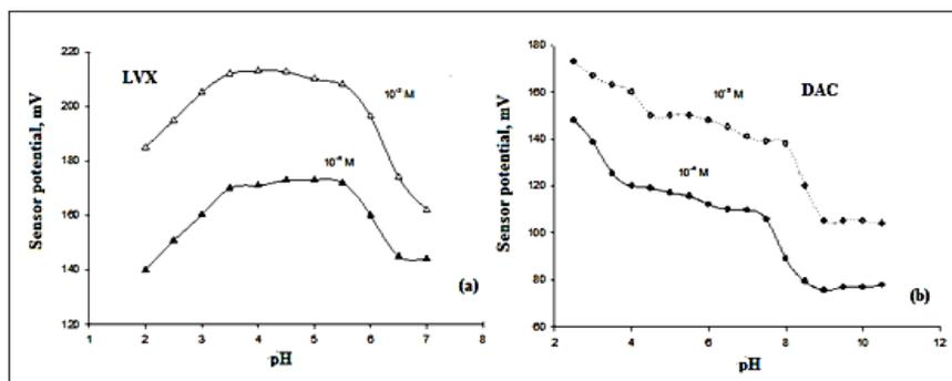
**Fig. 4. pH influence on LVX-TPB and DAC-TPB sensors**
