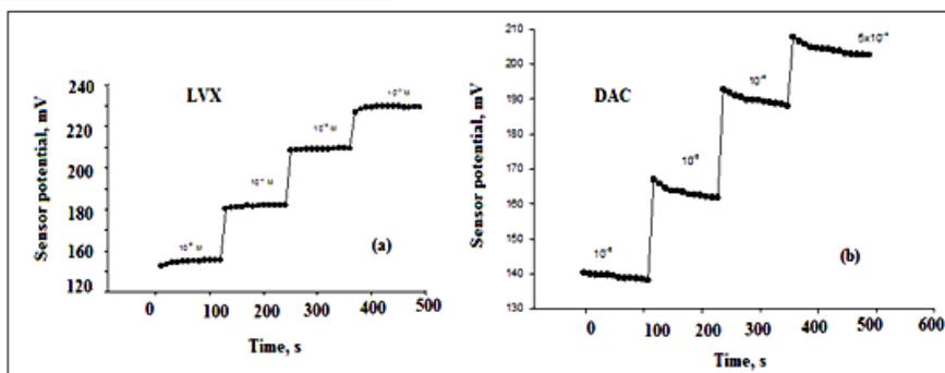
**Fig. 3. Response time plot for (a) LVX-TPB and (b) DAC-TPB membrane sensors**
