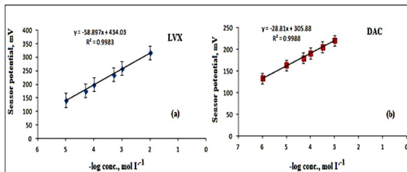
Figure 2: Typical calibration graphs of LVX-TPB and DAC-TPB plastic membrane sensors
