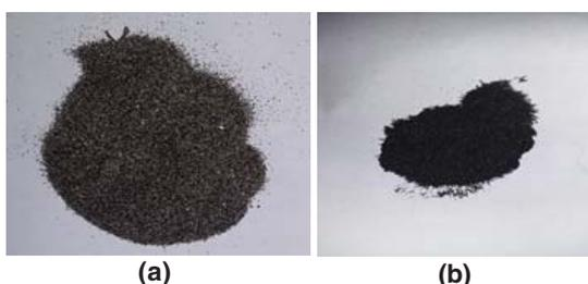
Fig. 1. The original iron sand from marina beach before extraction treatment with permanent magnet (A) Magnetite after extraction treatment
