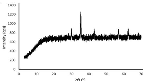
Fig. 3. Diffractogram XRD of magnetite after extraction treatment
