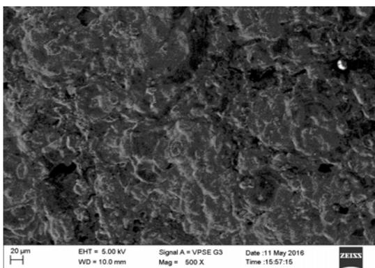
**Fig. 7. The SEM photo of mild steel when immersed in 1M HCl without inhibitor**
