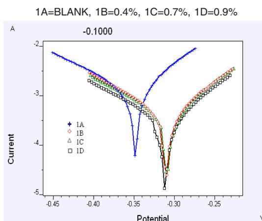
**Fig. 3. Potentiodynamic polarization technique diagram for mild steel in 1M HCL in the absence and presence of different concentrations of the inhibitor**
