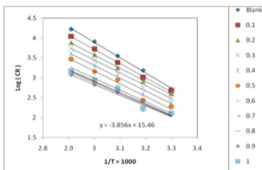
Fig. 5. Arrhenius plot for mild steel dissolution in 1M HCl from 303 K to 343 K temperature with and without inhibitor
