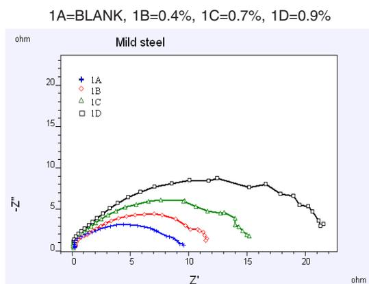
**Fig. 4. Impedance technique for mild steel diagram in 1M HCl in the absence and presence of different concentrations of the inhibitor**
