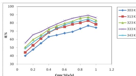
**Fig. 2. Gentamicin inhibitor Inhibition efficiency with various concentrations and temperatures****Table. 2: Effect of temperature on the corrosion of mild steel in the presence of difference concentration of Expired *Gentamicin* inhibitor in 1M HCL**
