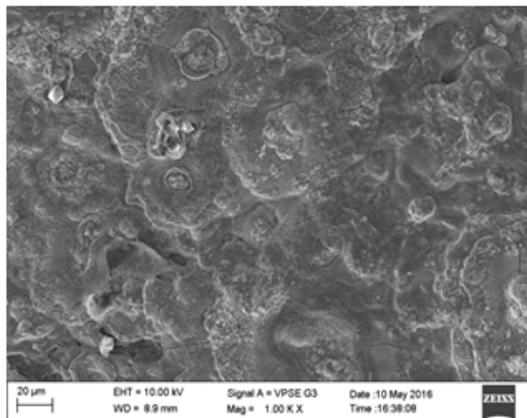
**Fig. 8. The SEM photo of mild steel when immersed in 1M HCl containing 0.9% concentration of inhibitor.**
