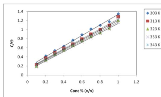
Fig. 6. Langmuir isotherm plot on mild steel surface in 1 M HCl solution for the adsorption of inhibitor
