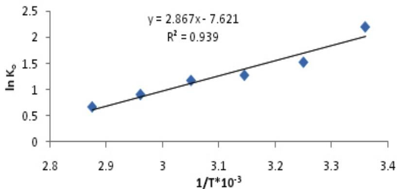
Fig. 3: The effect of temperature on equilibrium constant values ( $X_0=30$  mg.L<sup>-1</sup>, pH=7, MMPCL = 40 mg,  $t_c=50$  min).
