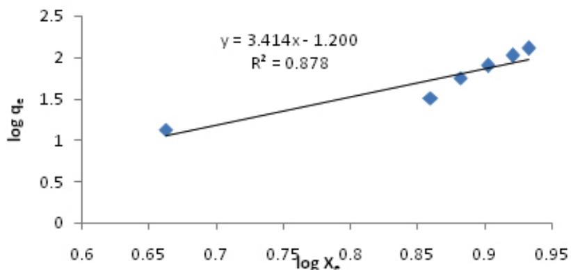
Fig. 1: Freundlich isotherm for cobalt ion adsorption onto MPCL (pH = 7,  $t_c=50$  min,  $T=298$  K, MMPCL = 40 mg).
