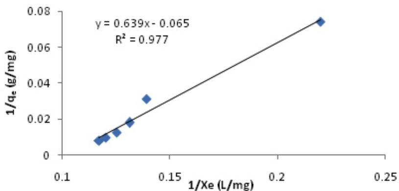
Fig. 2: Langmuir isotherm for cobalt ion adsorption onto MPCL (pH = 7,  $t_c=50$  min,  $T=298$  K, MMPCL = 40 mg).
