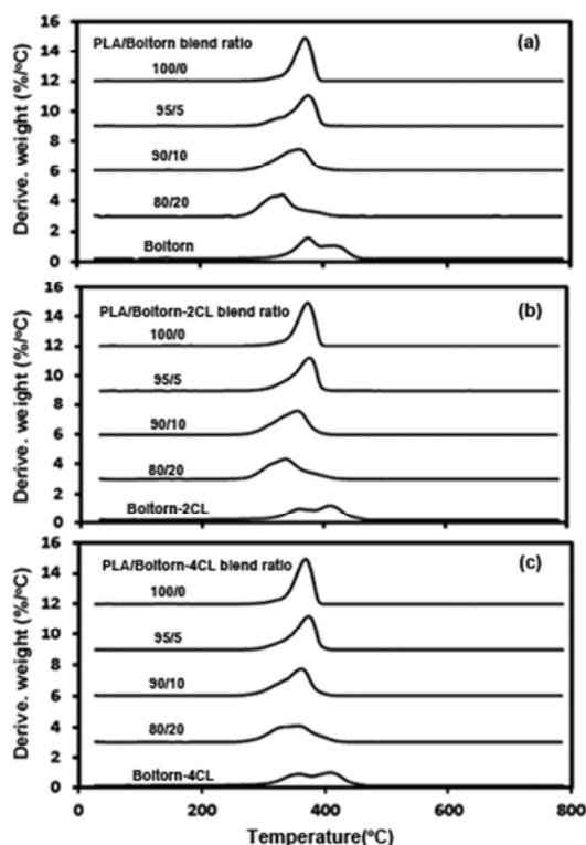
Fig. 6: DTG thermograms of (a) PLA/Boltorn, (b) PLA/Boltorn-2CL and (c) PLA/Boltorn-4CL blend films prepared with different blend ratios.
