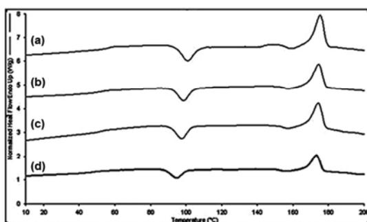
**Fig. 4:** DSC thermograms of (a) neat PLA, (b) 95/5 PLA/Boltorn, (c) 90/10 PLA/Boltorn and (d) 80/20 PLA/Boltorn blend films.
