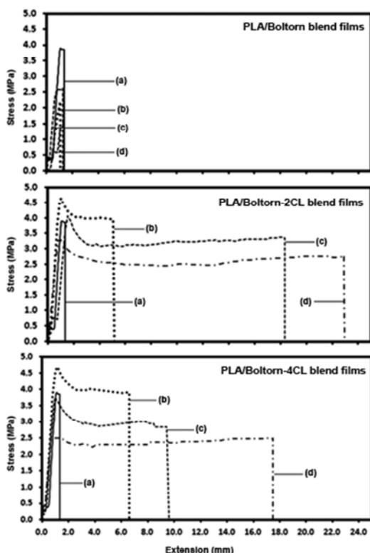
Fig. 7: Tensile curves of (a) neat PLA and PLA blend films prepared with PLA/plasticizer ratios of (b) 95/5, (c) 90/10 and (d) 80/20 wt%.
