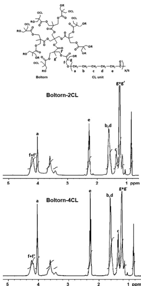
**Fig. 1:**  $^1\text{H-NMR}$  spectra of (above) Boltorn-2CL and (below) Boltorn-4CL in  $\text{CDCl}_3$  (peak assignments as shown).
