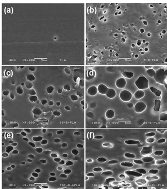
**Fig. 3:** SEM images of fractured surfaces of (a) neat PLA, (b) 95/5 PLA/Boltorn, (c) 90/10 PLA/Boltorn, (d) 80/20 PLA/Boltorn, (e) 80/20 PLA/Boltorn-2CL and (f) 80/20 PLA/Boltorn-4CL blend films (all bars = 5 mm).
