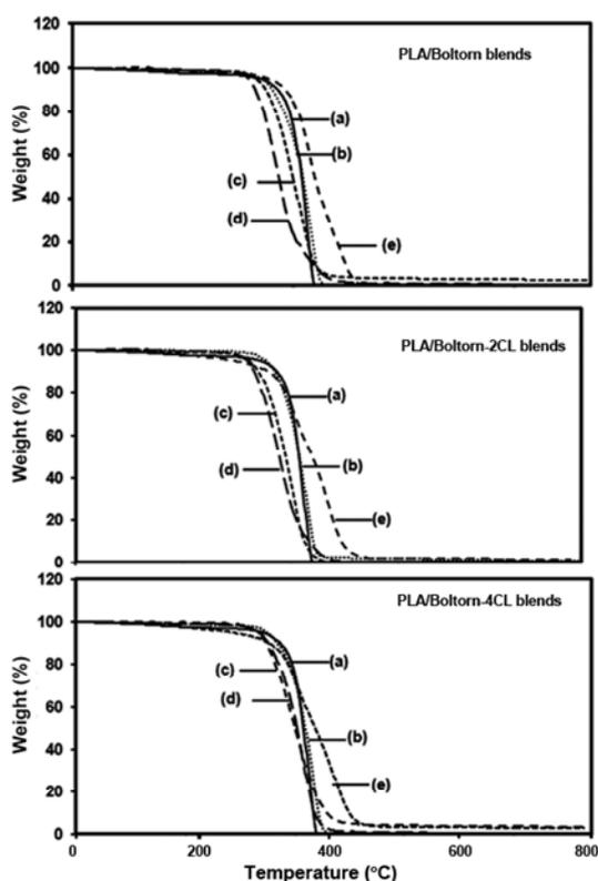
Fig. 5: TG thermograms of (a) neat PLA and PLA blend films prepared with PLA/plasticizer blend ratios of (b) 95/5, (c) 90/10 and (d) 80/20 (w/w) and (e) plasticizer.
