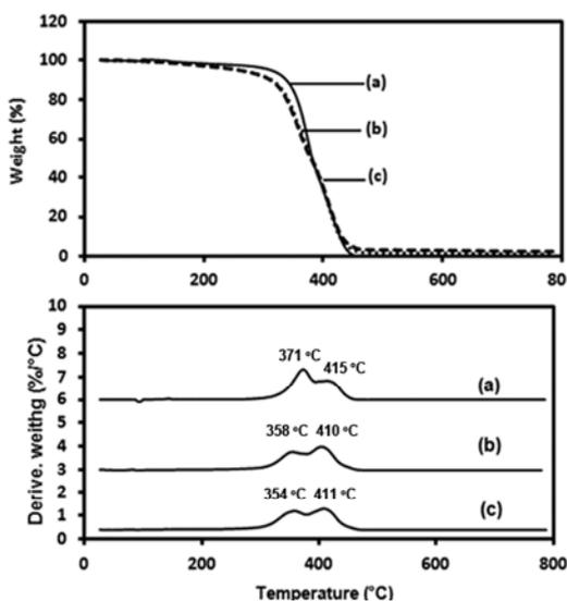
Fig. 2: TG (above) and DTG (below) thermograms of (a) Boltorn H2004, (b) Boltorn-2CL and (c) Boltorn-4CL.
