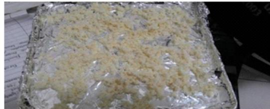
Fig. 2: Crushed  $\alpha$ -cellulose
