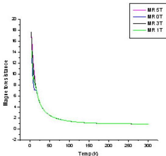
Fig. 3. The magnetoresistance (MR) of  $\text{La}_{1.8}\text{Ca}_{0.2}\text{Cu}_{0.85}\text{Mn}_{0.15}\text{O}_4$ .
