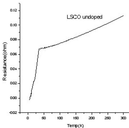
Fig 4. R-T plot for undoped LSCO.
