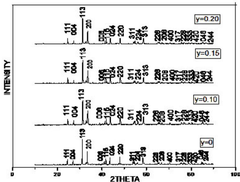
Fig 1. X-ray diffraction of LCCO i.e.  $\text{La}_{1.8}\text{Ca}_{0.20}\text{Cu}_{1-x}\text{Mn}_x\text{O}_4$  with  $x=0,0.10, 0.15,0.20$
