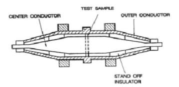
Fig. 5: Coaxial Transmission Line Method for SE measurement
