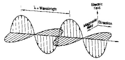
Fig. 1: Electromagnetic wave
