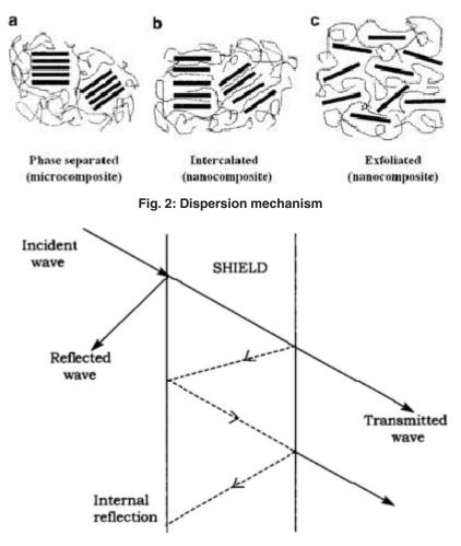
Fig. 3: Mechanism of EMI shielding
