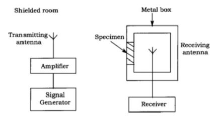
Fig. 4: Shielded Box and Shielded room Method for SE measurement
