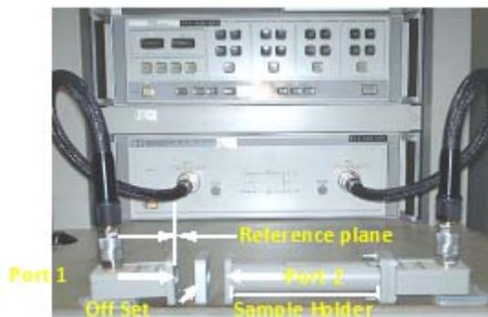
Fig. 3: Setup for measurements of S parameters
