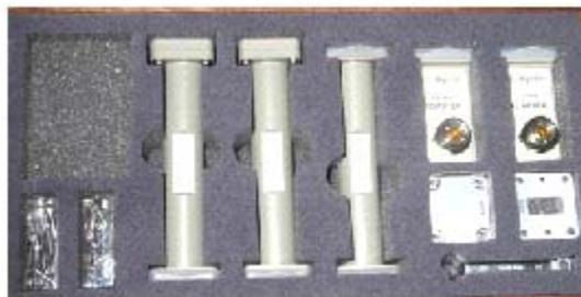
Fig. 2: Wavaveguide calibration set for X band
