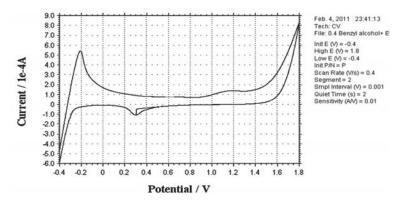
Benzyl alcohol + Ethanol + KOH on Pt working electrode
