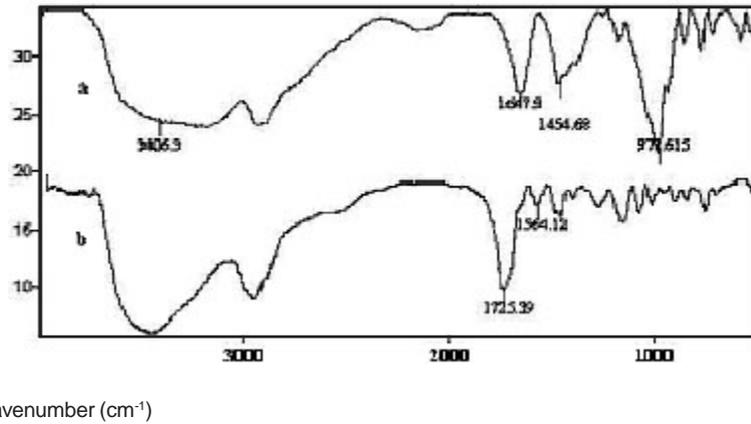
Fig. 2: FTIR spectra of (a) pure starch and (b) starch-g-(MAA-co-HEMA) hydrogel
