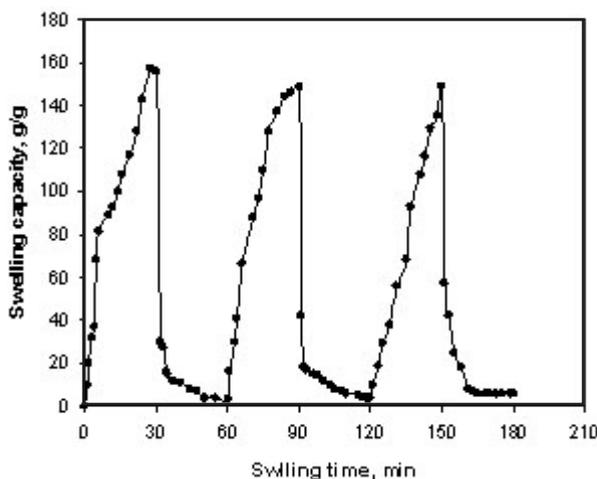
Fig. 6: On-off switching behavior as reversible pulsatile swelling (pH 7.4) and deswelling (pH 1.2) of starch-g-(MAA-co-HEMA) hydrogel
