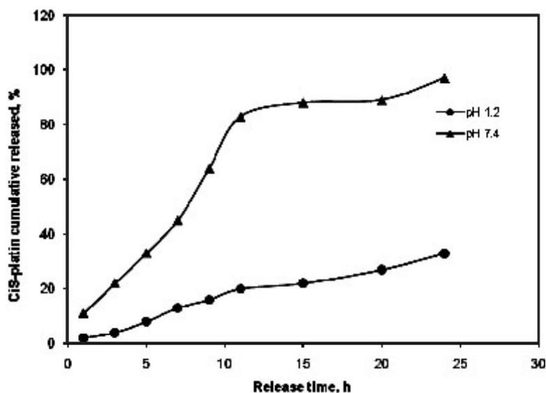
**Fig. 7: Release of Cis-platin from hydrogel carrier as a function of time and pH at 37°C**
