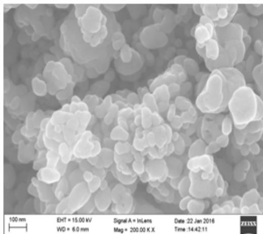
**Fig. 6c, 6d:** FE-SEM images of ZnO nanoparticles using 0.3% Al gum
