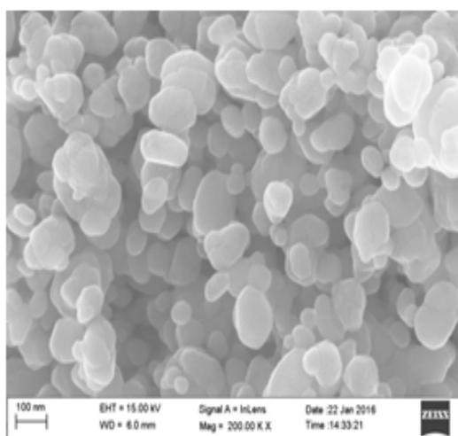
Fig. 5a, 5b: FE-SEM images of ZnO nanoparticles
