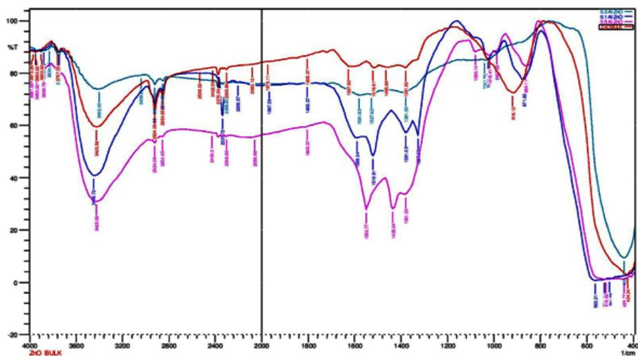
Fig. 3: FT-IR spectra of bulk ZnO and 0.1%, 0.3% and 0.5% Al gum stabilized ZnO nanoparticles
