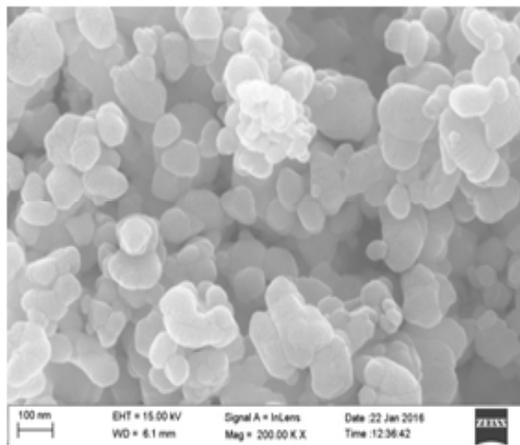
**Fig. 6a, 6b:** FE-SEM images of ZnO nanoparticles using 0.1% Al gum
