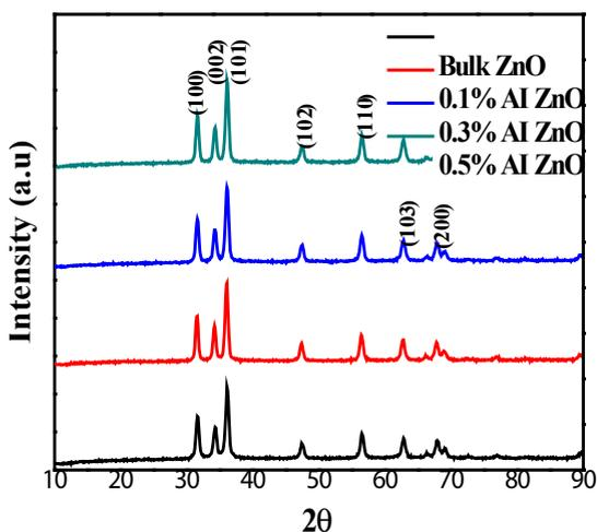
Fig. 4: XRD pattern of bulk ZnO and Al gum stabilized ZnO nanoparticles
