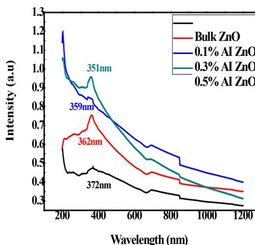
**Fig. 1: UV absorption spectra of bulk ZnO and Al gum stabilized ZnO nanoparticles**
