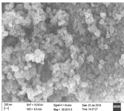
**Fig. 6e, 6f:** FE-SEM images of ZnO nanoparticles using 0.5% Al gum
