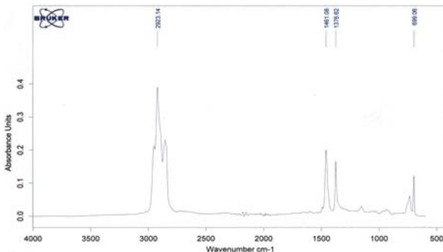
Fig. 1: The spectre IR of a copolymer Paratone 8900
