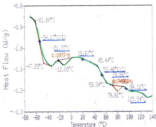
Fig. 2: The diagram DSC of a copolymer Paratone 8900
