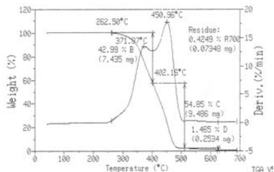
Fig. 3: The experimental TG and DTA curves for Paratone 8900
