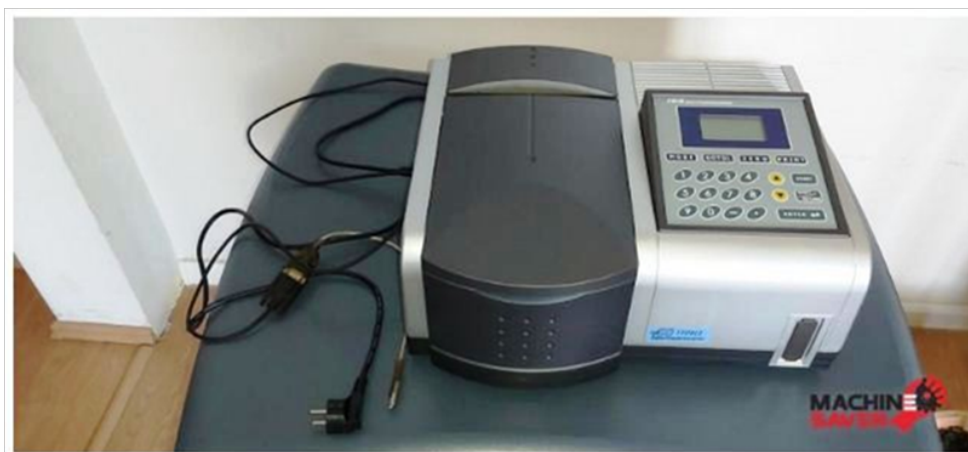
Fig. 1: T60V spectrophotometer used for spectral measurements
