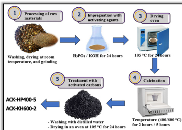
Fig. 2. Scheme of synthesis protocol for shea nut shells-derived activated carbons. (This work)
