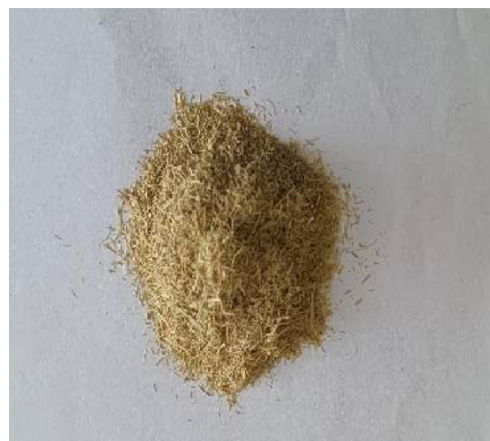
Fig. 2: Photograph of the CNF-Alkaline reinforcement
