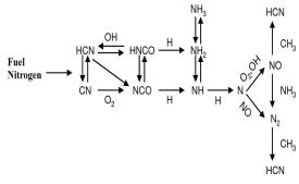
Fig.1. Mechanism of NO production from fuel nitrogen41
