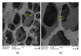
Fig. 8. SEM images of the cellular structure of HPCM: a - a general view of the honeycomb frame structure, b - a jumper
