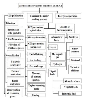
Fig. 3. Methods for reducing the toxicity of exhaust gases (EG) from internal combustion engines (ICE)<sup>51</sup>
