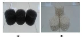
Fig. 9. A blank of polyurethane foams 20 ppi (a), a sample of HPCM (b)
