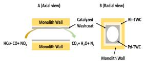
Fig. 5. A washcoated monolith automotive three-way-catalyst62
