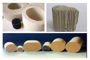
Fig. 7. General view of ceramic block carriers<sup>66</sup>
