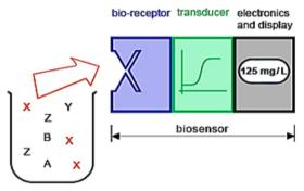
Fig. 1. Components of a Biosensor, Modified from: https://www.ufz.de/index.php?en=39398
