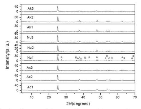
Fig. 2: X-ray difractograms of  $TiO_2$  samples calcined at 550°C. A= anatase and R = rutile
