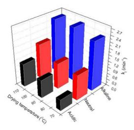
Fig. 6: The Calculated rate constants of the hydroxylation of coumarin using different TiO<sub>2</sub> samples
