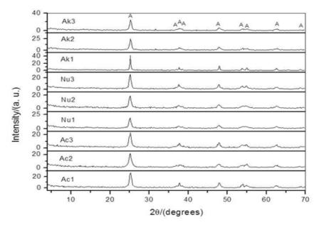
Fig .1: X-ray difractograms of TiO<sub>2</sub> samples calcined at 450 °C. A= anatase
