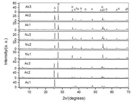
Fig. 3: X-ray difractograms of TiO<sub>2</sub> samples calcined at 650°C. A = anatase and R = rutile
