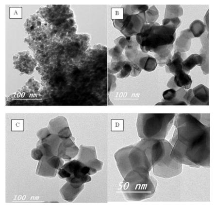
Fig. 4: TEM micrographs of TiO<sub>2</sub> nanoparticles prepared at different experimental conditions. A: Nu1 at 450 °C, B: Nu3 at 550 °C, C: Ac2 at 650 °C, and D: Nu1 at 650 °C
