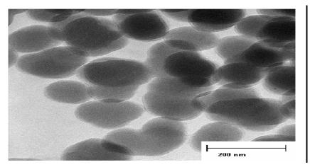
Fig. 10: Transmission Electron Microscope image of Silica nanoparticles
