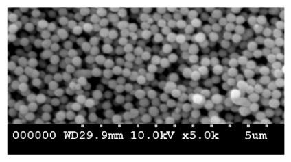
Fig. 9: Scanning Electron Microscope image of Silica nanoparticles
