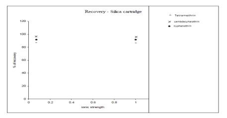
Fig. 7: Influence of ionic strength in pre-concentration of pyrethroid residues
