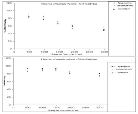
Fig. 5: Effect of sample volume in pre-concentration of pyrethroid residues
