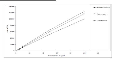
Fig. 1: Calibration of pyrethroids using GC-EI-MS
