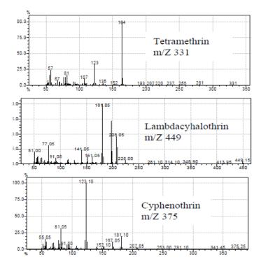
Fig. 3: GC-EI -MS mass spectra of pyrethroids
