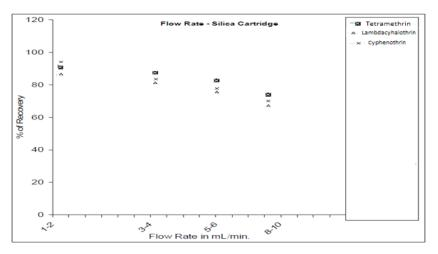
Fig. 4: Effect of flow rate in pre-concentration of pyrethroid residues
