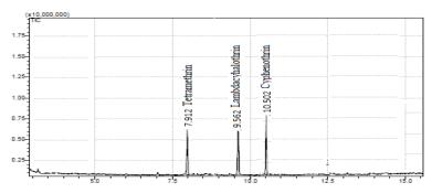
Fig. 2: Representative GC-EI-MS total ion chromatogram recovery of pyrethroids by using silica nanoparticles cartridge
