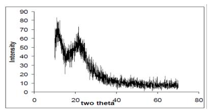
Fig. 11: XRD patterns of Silica nanoparticles
