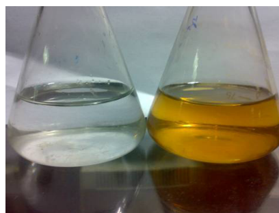
Fig. 1: Colour change of silver nitrate 1mM solution from colourless to yellow brownish as the reaction proceeds on addition of the culture supernatant
