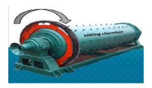
Fig. 1: A rock tumbler Ball mills (reprinted from Ref. 12)
