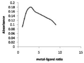
Fig. 4: Jobs method for Cr(III)-2,6PDC complex
