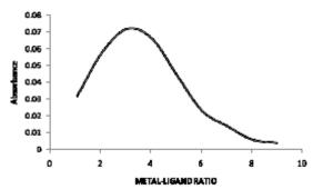
Fig. 6: Jobs method for Cr(III)-2,5PDC complex
