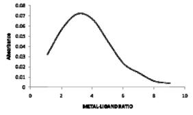
Fig. 5: Jobs method for Cr(III)-2,3PDC complex
