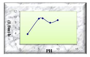
Fig. 1: Effect of pH on the removal of Pb(II)
