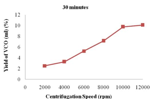
Fig. 2: Results of VCO yield (%) under different centrifugation speed (rpm) at 30 min
