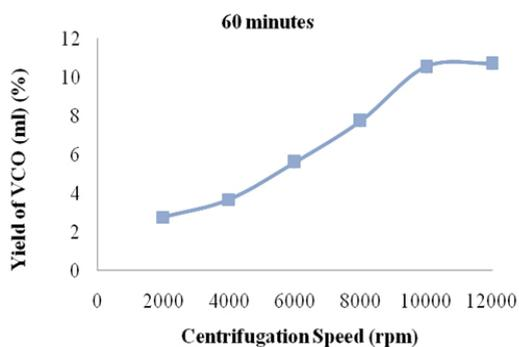
Fig. 3: Results of VCO yield (%) under different centrifugation speed (rpm) at 60 min
