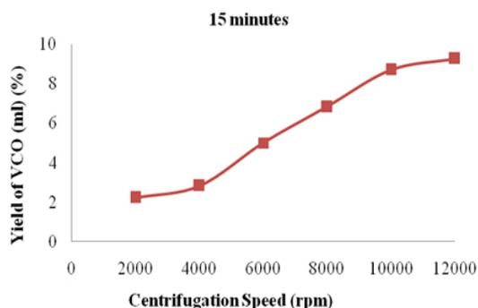
Fig. 1: Results of VCO yield (%) under different centrifugation speed (rpm) at 15 min
