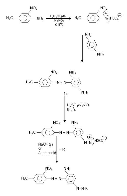
Scheme 1: Synthesis of Disazo dyes derived from 4-amino-3-nitrotoluene
