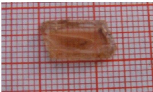
Fig. 2: As grown crystals of N' -[( E )-(4-Bromophenyl)(phenyl)methylidene]-4-methylbenzenesulfonylhydrazide
