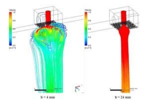
Fig. 7: Outdoor air flow lines without recirculation
