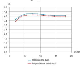
Fig. 9: Velocity coefficient *m* - relative distance graph
