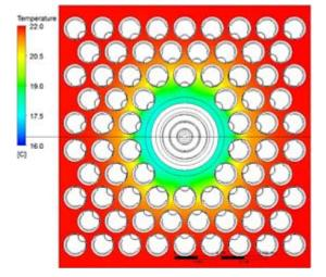
Fig. 6: Temperature field on the air diffuser panel
