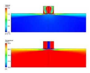
Fig. 5: Velocity and air temperature fields on the vertical plane
