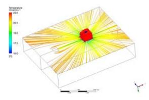
Fig. 4: Air flow lines at the local recirculation diffuser outflow
