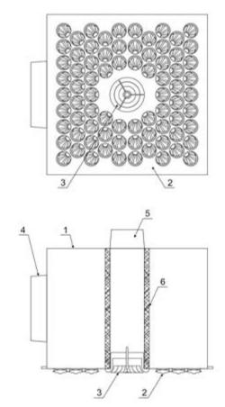
1 - plenum chamber, 2 - face plate, 3 - diffuser, 4 - feed duct for recirculation air, 5 - feed duct for intake air, 6 - heat insulation.
