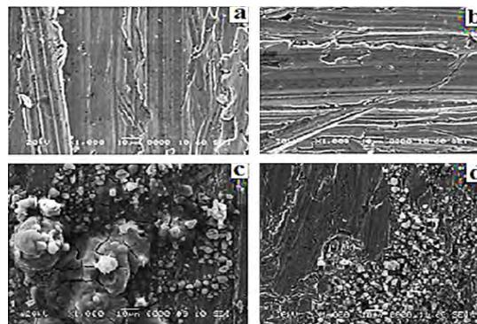
**Fig. 11. SEM of (a) MS in HCl (b) MS in  $\text{H}_2\text{SO}_4$  (c) MS in HCl + inhibitor (600ppm) (d) MS in  $\text{H}_2\text{SO}_4$  + inhibitor (600ppm)**
