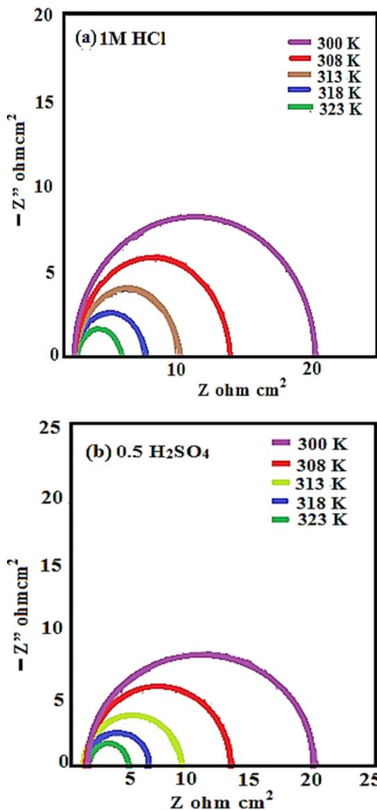
Fig. 8. Nyquist plots of MS in NB4MA of (a) 1M HCl (b) 0.5M H<sub>2</sub>SO<sub>4</sub>
