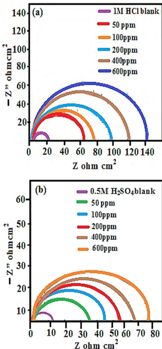
Fig. 7. Nyquist plots of MS in NB4MA (a) 1M HCl (b) 0.5M H<sub>2</sub>SO<sub>4</sub>
