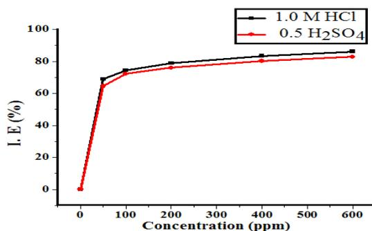
**Fig. 5. Corrosion inhibition effectiveness of NB4MA**
